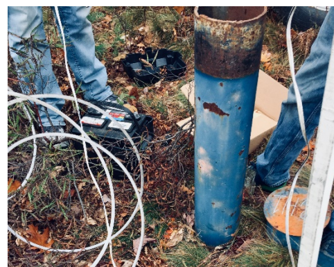
Figure 2. Well head at the Deblois 2 site with sounding tape, HDPE tubing, post-sample extraction and pre-decontamination.
