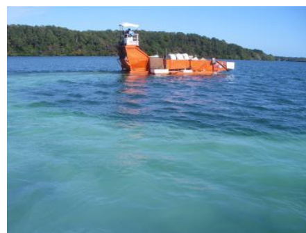
A barge applying aluminum on a lake. (Photo: WRS, Inc.)
