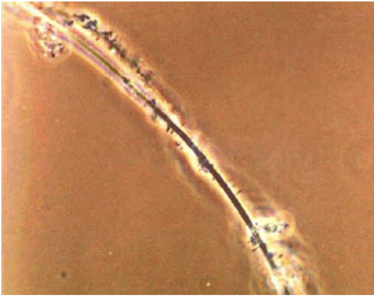
Photomicrograph of type 0041. Notice attached growth typical of type 0041.
