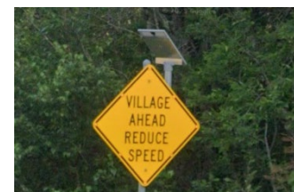
Wayne - Route 133 Flashing LED "Village Ahead Reduce Speed" Sign
